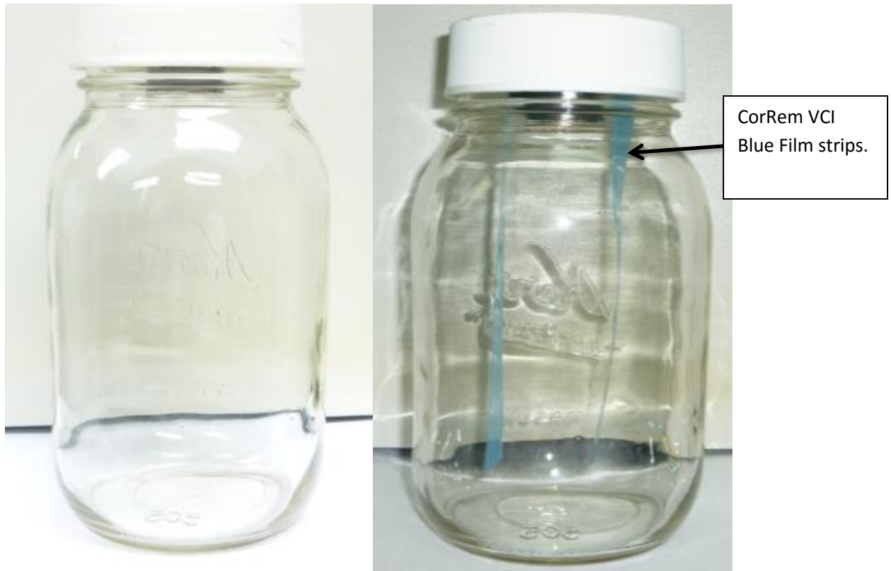
Figure 2. Jars set for corrosion testing: Blank (left), VCI Film (right)
