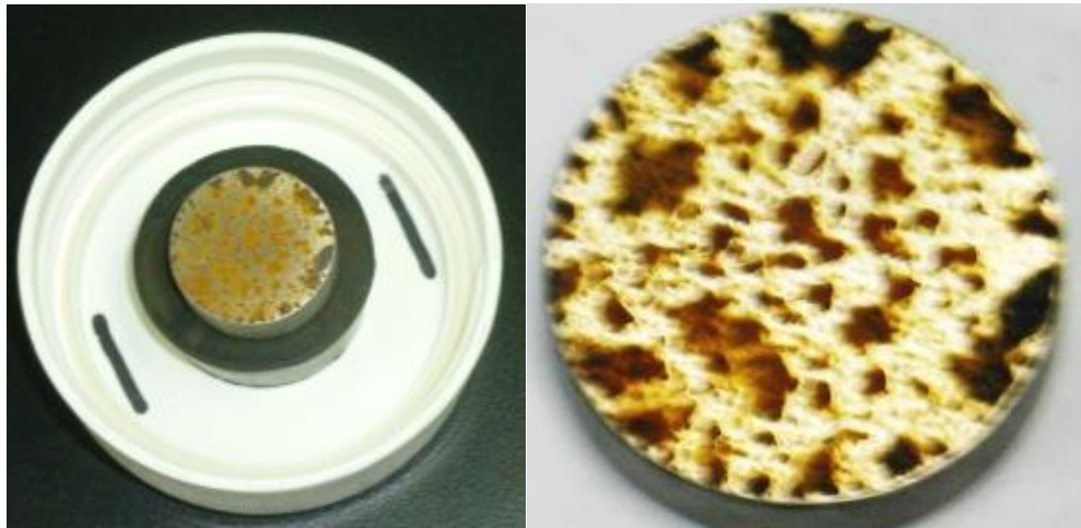
Figure 4. No corrosion protection effect (Blank)
