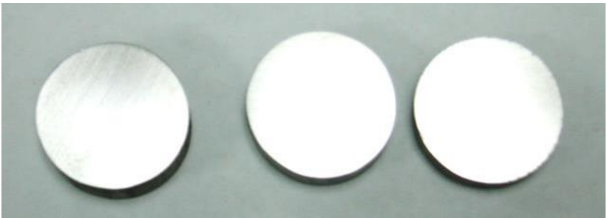
Figure 5. Performance of the CorRem VCI Film: GOOD corrosion inhibiting properties
