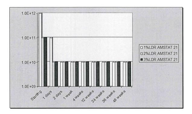
Note: Film samples are made with AMSTAT 21 in 30 μm LDPE Blown film Surface resistivity measured at 50%RH, 25°C
